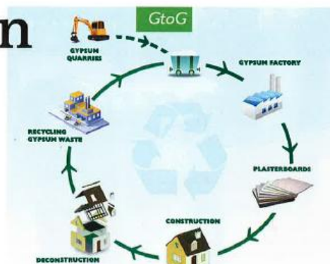
Gypsum in a closed loop system
